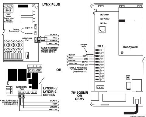
Figure 3. 7845GSMR or GSMV Connections
